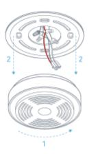
**Note**: If you don't have an old smoke alarm, skip to step 9. To prevent electrical shock, make sure the green power light is off on the alarm. You may have to twist the alarm to release it. Carefully remove it to keep from damaging your ceiling or wall.
