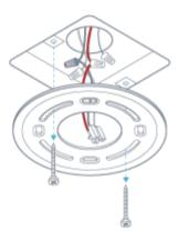
Unscrew the backplate from the electrical box. Save the screws to install the Nest Protect backplate later.
