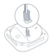
Plug the 120V connector into the back of your Nest Protect.
