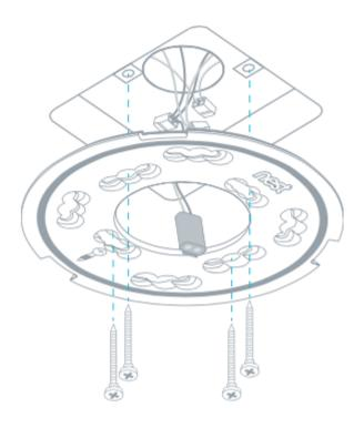
Screw the Nest backplate to the existing electrical box, reusing the existing screws. You can also screw the backplate directly into the wall or ceiling with the Nest screws.
