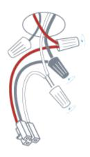
Twist the wire connectors counterclockwise to unscrew them and detach the 120V connector from your old smoke alarm.
