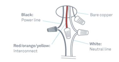
Hold the white wire ends together, cap them with a wire connector and twist clockwise until it's secure. Do the same with the black wires. If there are any extra wires, you won't need them. Cap them with wire connectors.
